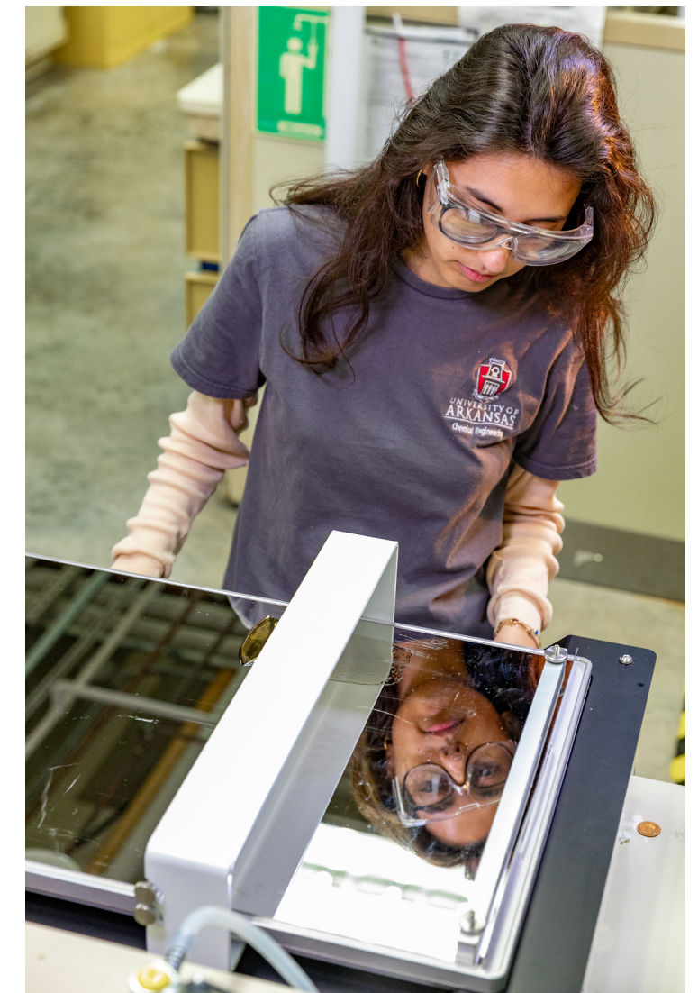
Doctoral student Juliana Marcal works with a membrane caster, a machine used for making sheet membranes.
